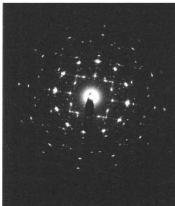
Figure 4. Selected area electron diffraction pattern of an InSe film grown at 350 °C using [(\text{Bu})_2\text{In}(\mu\text{-Se}^t\text{Bu})_2] .
